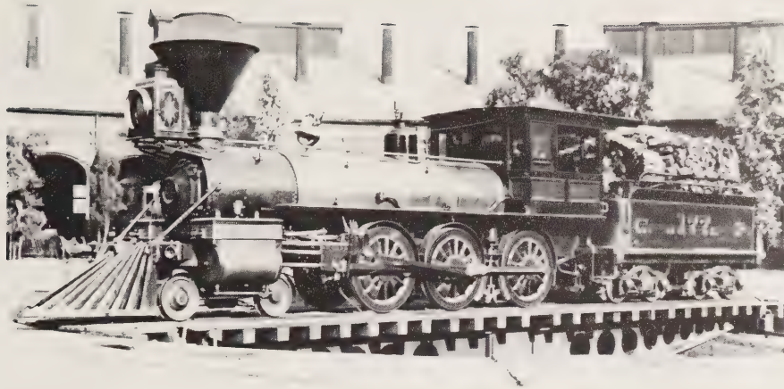
Ten-wheeled (4-6-0) Type, with Stevens Valve Gear, Built at Sacramento in 1887 Cylinders 18" x 30" Steam pressure 145 lb. Heating surface 1,453 sq. ft. Drivers, diam. 57" Grate area 24.5 sq. ft. Tractive force 21,020 lb. Weight on drivers 78,700 lb. Weight, total engine 105,100 lb.
